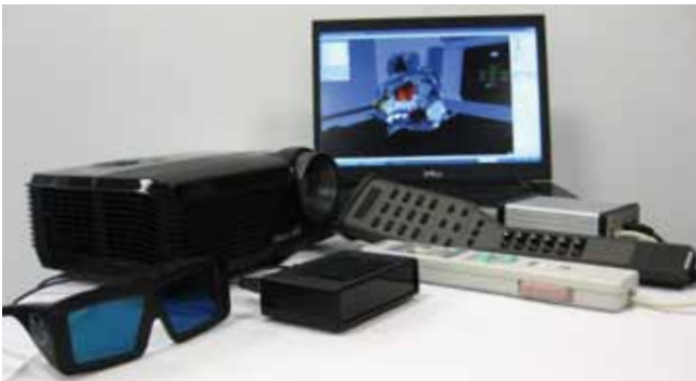
Below: Recruitment VERT™ equipment, namely: 3D projector, laptop, 3D glasses, actual pendants for controlling virtual radiotherapy treatment machine.
