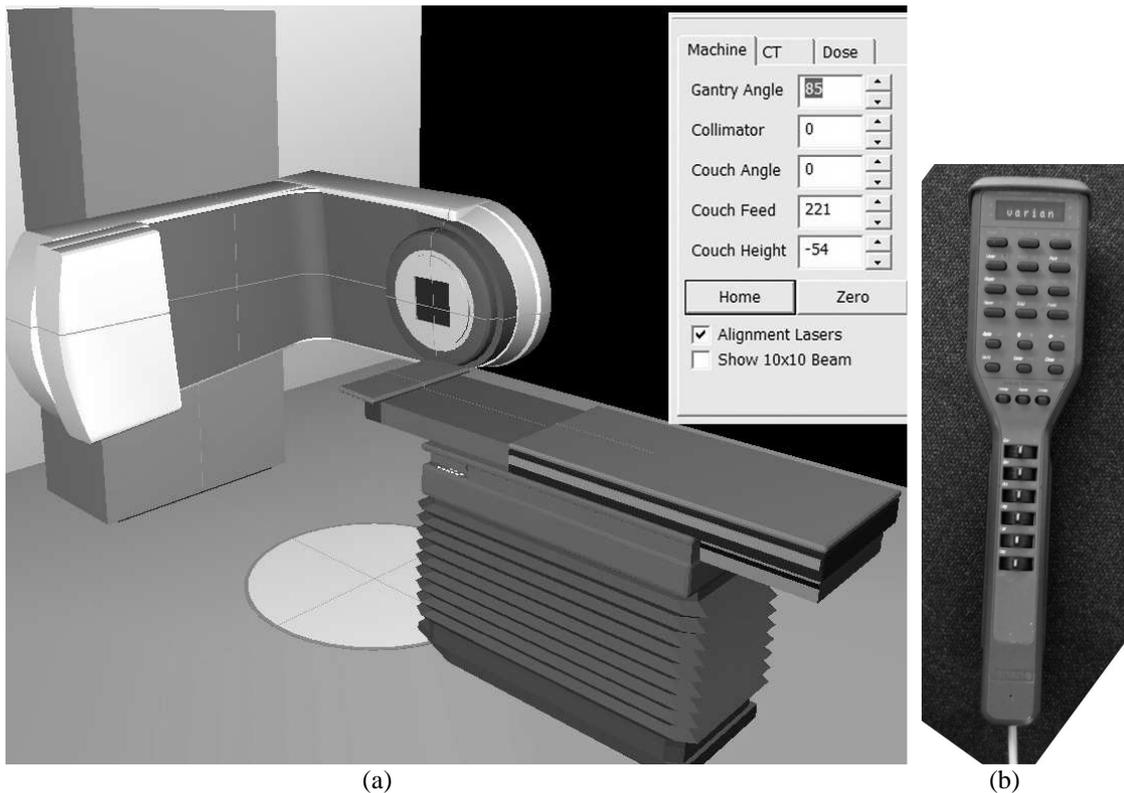
**Fig. 1.** (a) Virtual linear accelerator, couch and alignment lasers (used for positioning the patient). Inset is the dialogue box for manual manipulation of the gantry and couch of the VE linear accelerator. Actual handset (b) that is being adapted for control of the VE linear accelerator.
