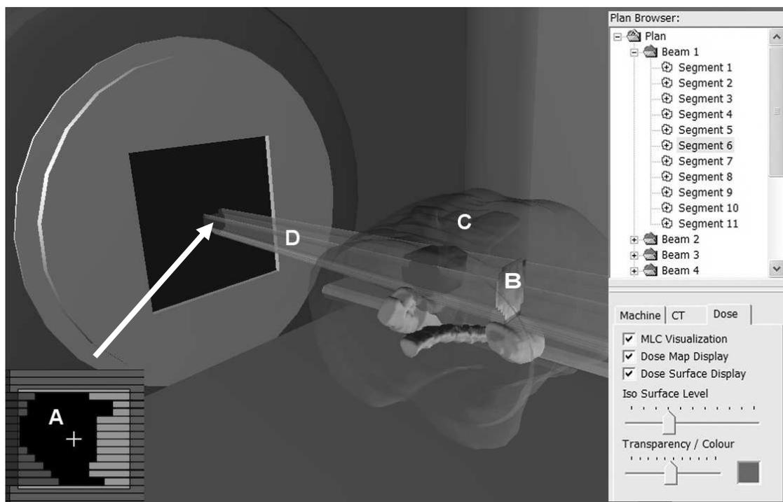
**Fig. 3.** Visualization of the radiation treatment. (D) visualization of segment 6 of treatment beam 1. The segment is shaped using a MLC inside the gantry head. (A) shows the leaf positions of this MLC. (B) dose map of the radiation intensity for beam 1. (C) dose isosurface showing the tissue volume that receives at least 30% of the maximum dose level. Inset is a dialogue box of dose visualization options.
